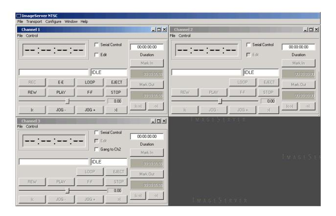
6. From the Menu Bar select <u>Configure / System ... / Control Tab</u> and select **VDCP** as the Serial Protocol for the channels connected to the Fastrack.
